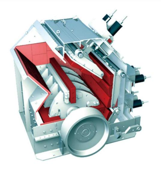
Impact crusher is widely used in the industry of road construction, building, , construction waste recycling, etc. The output material is cubic and suitable for railway and high way construction. The main parts are blow bar (impact hammer), impact plate and liner plate. Denp machinery produce high quality impact crusher parts including blow bar, impact plate and liner plate.
